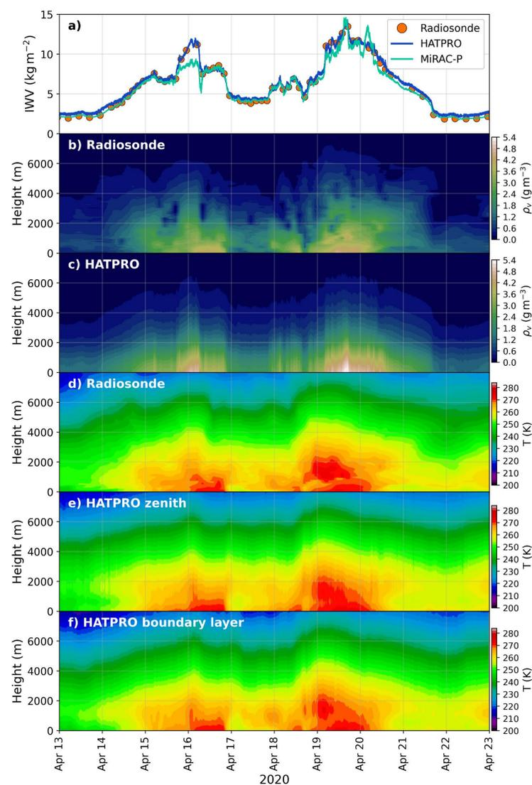
Fig. 4: Overview of moist air intrusion case from 13th to 23rd April 2020, showing IWV, absolute humidity and temperature profiles from **HATPRO**, **MiRAC-P** and radiosondes.
