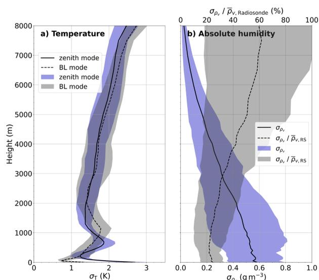
Fig. 3: Standard deviation of temperature and humidity profiles between radiosondes and those from **HATPRO**. Shading indicates the spread over the MOSAIC legs.
