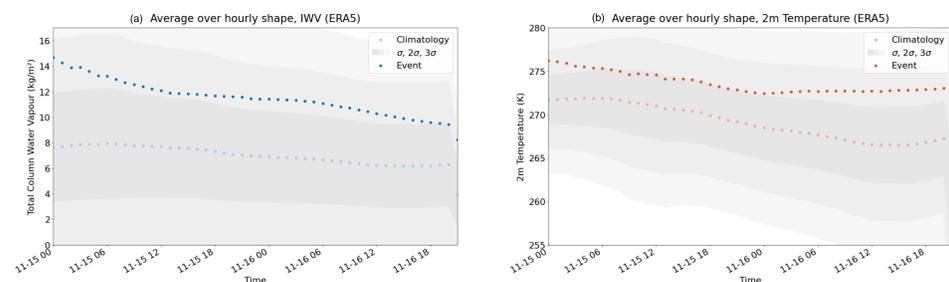
Fig 2: Climatological context of the events (a) integrated water vapor and (b) 2m temperature of the event. Values are averages over the hourly AR shape as detected by the algorithm using ICON data of the event. Darker color: event (ERA5), light color: climatology (ERA5). Grey ranges denote  $\sigma$ ,  $2\sigma$  and  $3\sigma$  range.
