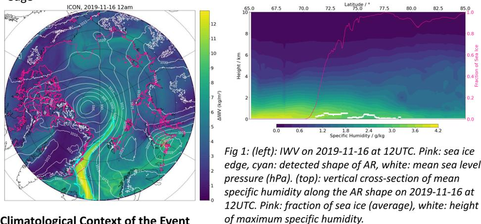
Fig 1: (left): IWV on 2019-11-16 at 12UTC. Pink: sea ice edge, cyan: detected shape of AR, white: mean sea level pressure (hPa). (top): vertical cross-section of mean specific humidity along the AR shape on 2019-11-16 at 12UTC. Pink: fraction of sea ice (average), white: height of maximum specific humidity.
