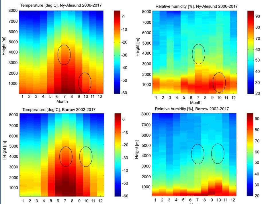
**Fig. 3:** Annual cycle of tropospheric temperature (left) and relative humidity (right) from radiosonde observations at Ny-Alesund from 2006 to 2017 (upper panels) and at Barrow from 2002 to 2017 (lower panels). Ellipses show altitudes with high occurrence of ice-containing clouds in July and October (see Fig. 2).
