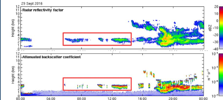
**Fig. 4:** Example of single-layer clouds, Ny-Alesund, 29 Sept 2016. Shown are the radar reflectivity factor (upper panel) and lidar attenuated backscatter coefficient (lower panel) from Cloudnet [2].
