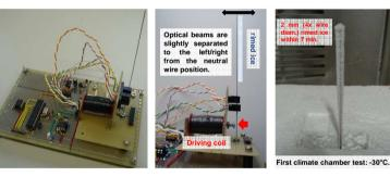
>The wire is given only a short impulse from the driving coil when it is moving towards the coil and crossing the two optical beams which are slightly horizontally separated. This ensures minimal influence on the resonance frequency.
