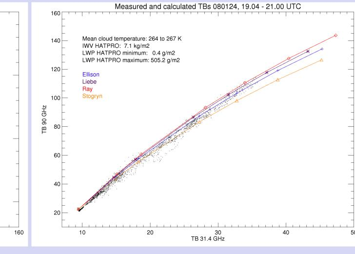
Thin single layer clouds are identified by ceilometer and cloudradar; Scatterplots of measured TB (black dots) are shown for 150/90 GHz (left) and 90/31.4 GHz (right). The colored lines represent the possible TB-range based on the different RI-models: Ellison2006, Liebe1991/93, Ray1972, Stogryn1995.
