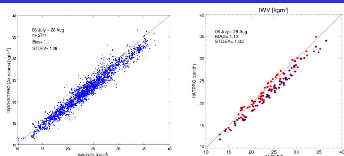
**Left:** Spatially averaged IWV from azimuth scans compared with GPS-Station at supersite M (operated by GFZ-Potsdam).
