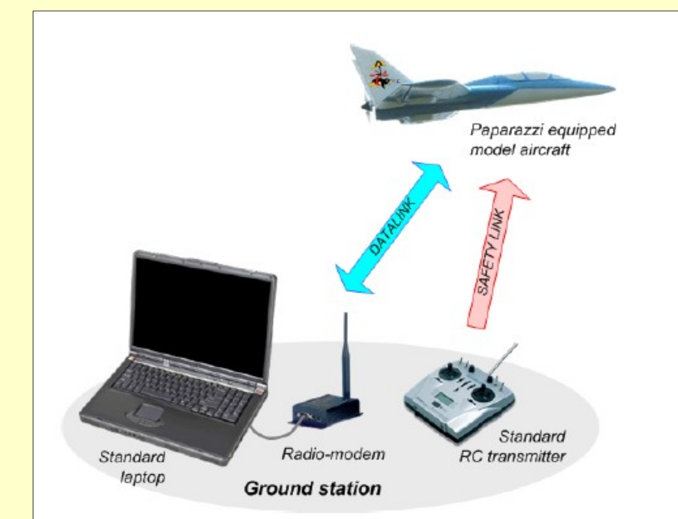
Figure 4: The Paparazzi system consists of the following four main components: An airborne part, a ground station, a radio modem and a safety remote control transmitter.
