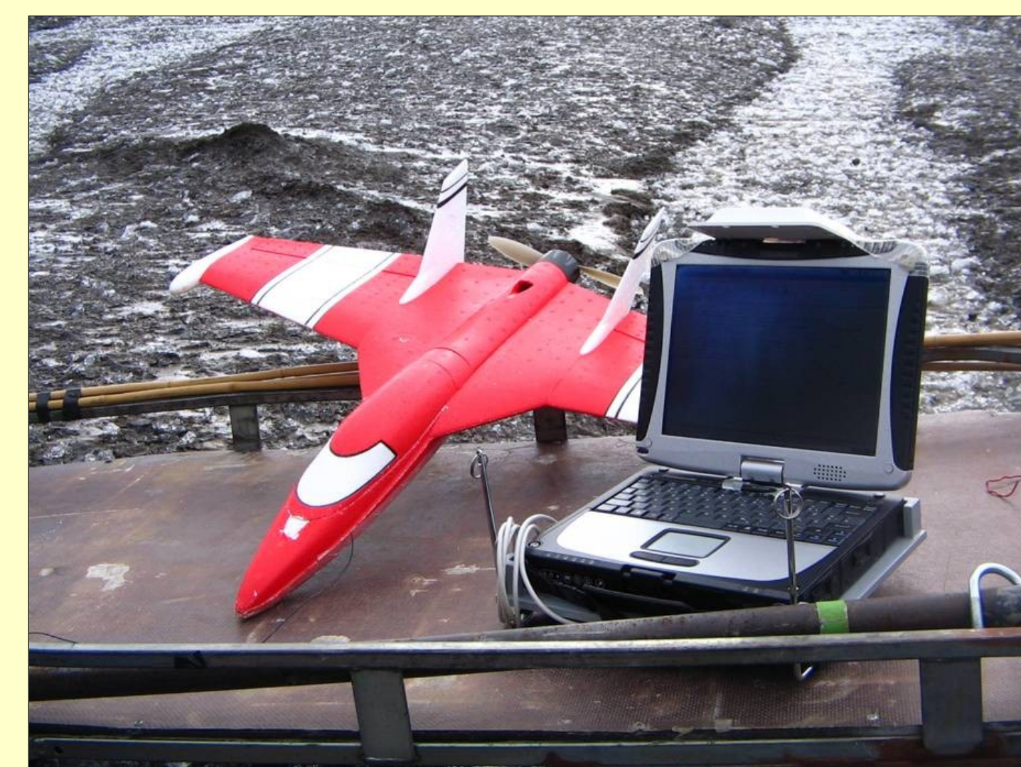
Figure 3: The SUMO aircraft and the laptop used as ground control station during operations.
