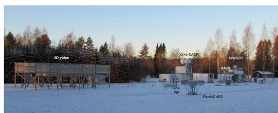
Figure 1: Instrument configuration during the ARM-BAECC campaign (winter 2014).
