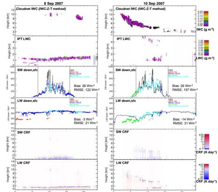
Fig. 6: Profiles of IWC and LWC for the days shown in Fig. 2: September 8 (left) and 10 (right), 2007. The observed and modelled downwelling surface fluxes and the calculated shortwave (SW) and longwave (LW) cloud radiative forcing (CRF = HR<sub>cloudy</sub> - HR<sub>clear</sub>) are also shown.
