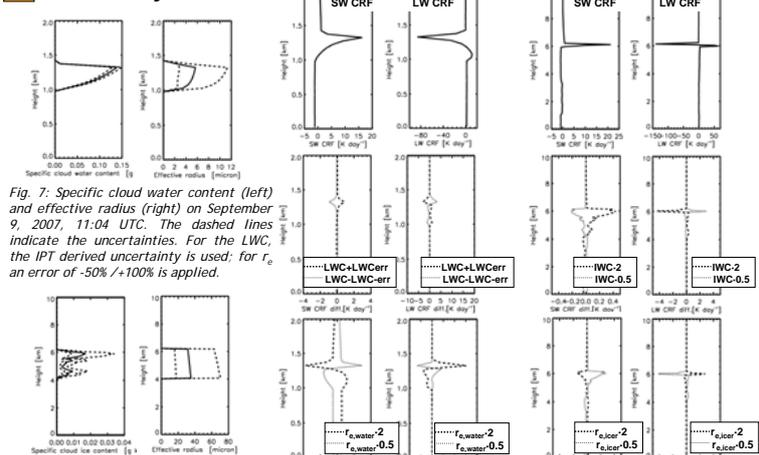
Fig. 7: Specific cloud water content (left) and effective radius (right) on September 9, 2007, 11:04 UTC. The dashed lines indicate the uncertainties. For the LWC, the IPT derived uncertainty is used; for  $r_e$  an error of -50% / +100% is applied.
