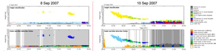
Fig. 3: Examples of the target classification product for the AMF site in the Black Forest: September 8 (left) and 10 (right), 2007. Cloudnet Target Classification (top) and radar/lidar detection status (bottom).
