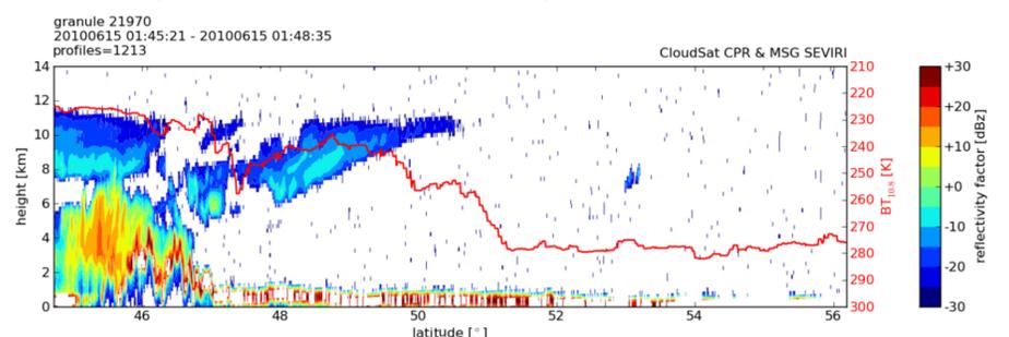
Cross-section of an A-Train overflight on 15 June 2010 02UTC CloudSat CPR radar reflectivity factor and MSG SEVIRI brightness temperatures as red line
