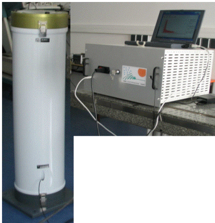
Figure 3 : view of the CAML emission-reception telescope, acquisition rack and 12" portable computer used for acquisition and control.
