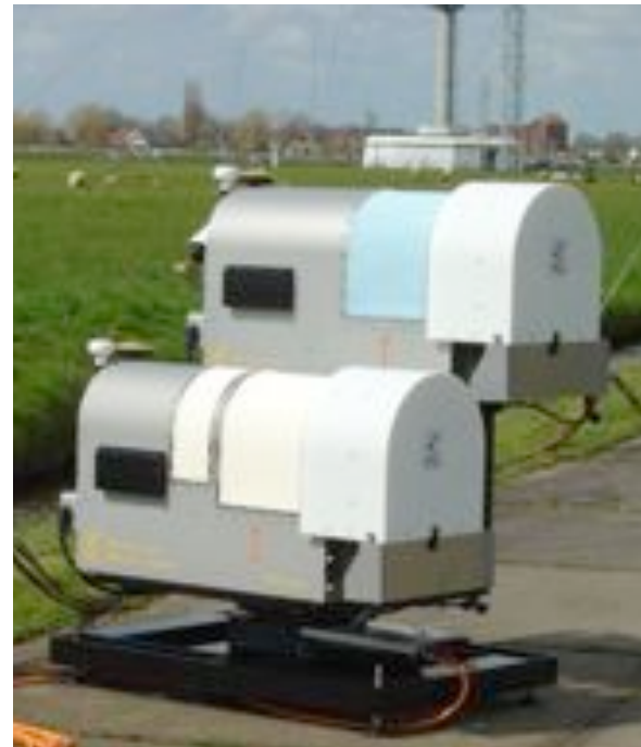
Fig. 1. ATPROP during the test campaign at the remote sensing site of Cabauw, The Netherlands. The radiometer unit in the back is a HATPRO and the lower unit in the front contains the 15.3 GHz (larger window) and 90 GHz (smaller window) radiometer.
