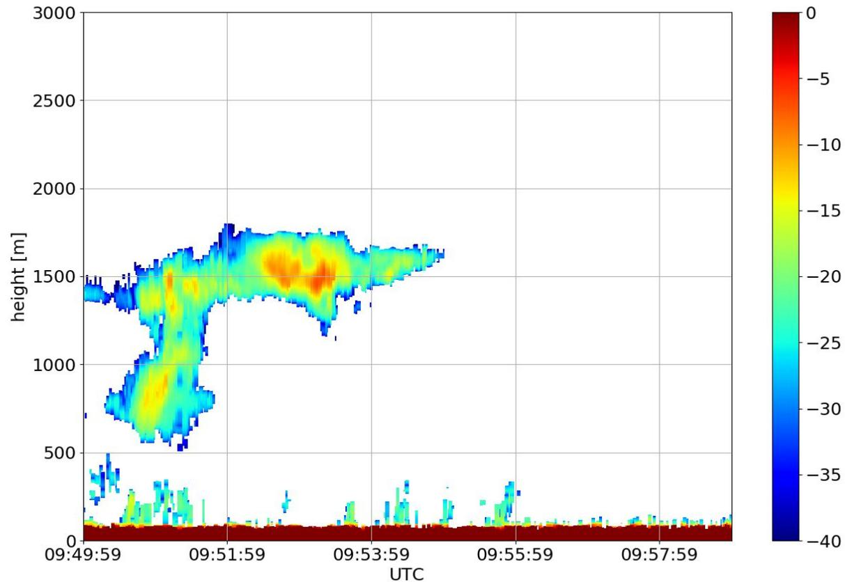
Filter detected signals for artifacts due to FMCW method, "mirrored" signal at surface, and clutter
