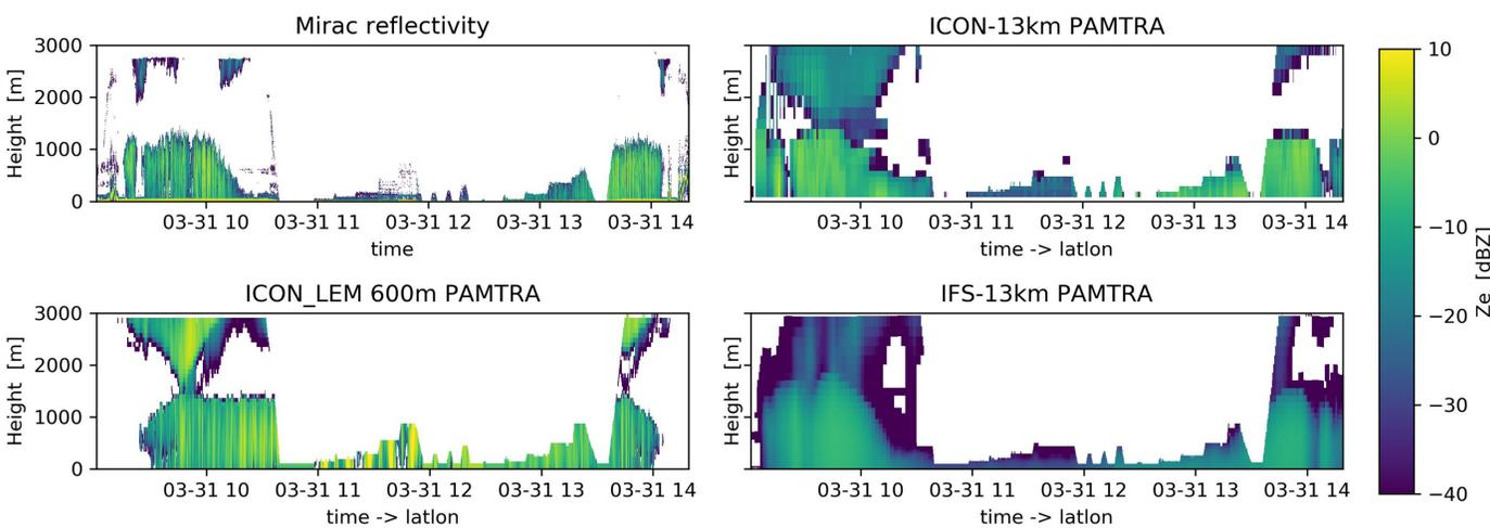
Fig. 2: The radar measurements (top-left panel) are compared with the simulated radar reflectivity along the flight track. The higher resolution of the **ICON-LEM** (bottom-left) allows to see the horizontal variability of the clouds simulated reflectivity values are closer to the observations.
