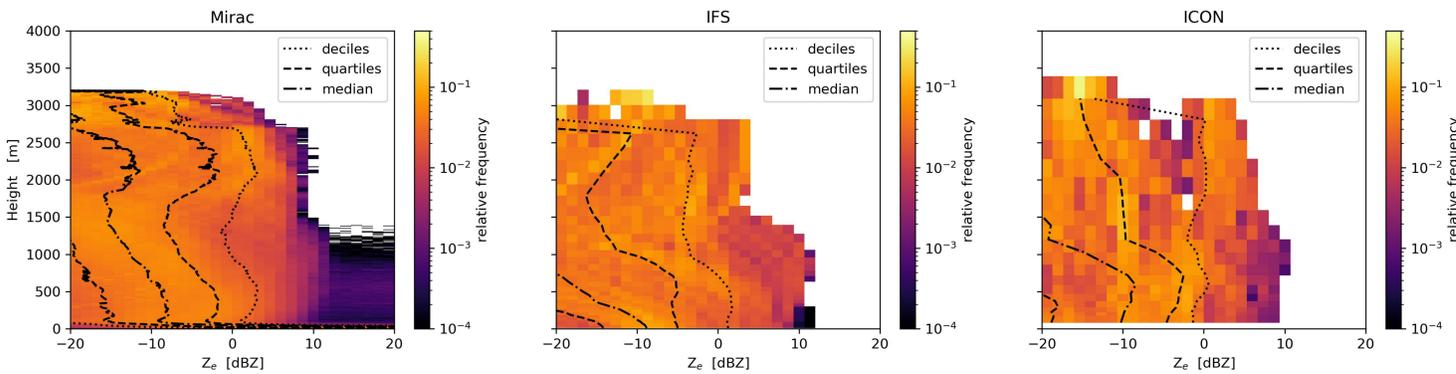
Fig. 2: Contoured Frequency Altitude Diagram (CFAD) of measured and simulated reflectivity. The distribution of simulated **Z** is well matched at the surface (precipitation rate is good) but the models tend to predict **too low reflectivity at higher levels**.
