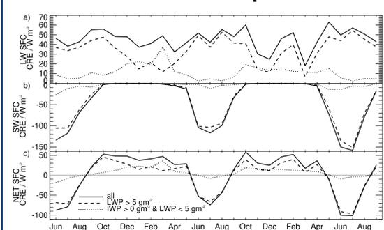
Fig. 7: a) LW, b) SW and c) net monthly mean SFC CRE for all conditions (solid line), for cases with  $LWP > 5 \text{ gm}^{-2}$  (dashed line) and for cases with  $IWP > 0 \text{ gm}^{-2}$  and  $LWP < 5 \text{ gm}^{-2}$  (dotted line). The grey solid line in c) indicates the zero line.
