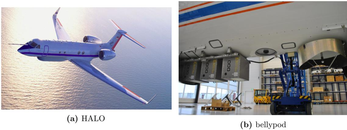
**Figure 3.2** – (a) HALO with NARVAL-South instrumentation (DLR [2006b]). (b) Bellypod instrumentation, from left to right: HAMP-G, HALO-KV, HALO-WF modules, WALES lidar and MIRA cloud radar (Mech et al. [2014])
