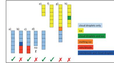
**Figure 2.** Examples for different possible Cloudnet cloud classifications in the atmospheric column where IPT currently is and is not applied.
