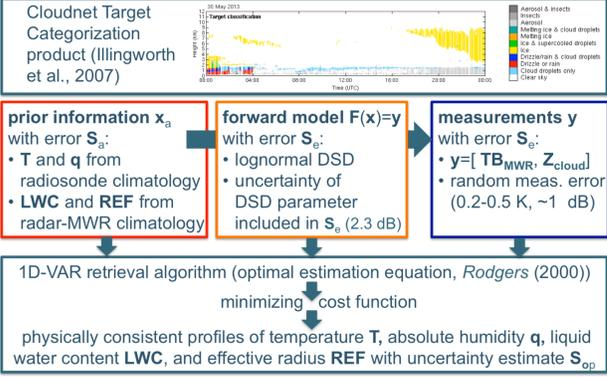
**Figure 1.** Schematic of the IPT. The IPT has been recently extended to also retrieve profiles of droplet effective radius (REF) including updated prior information on LWC and REF and a new forward model for Z.
