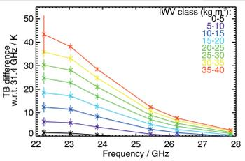
**Figure 8.** Mean TB differences between the lowest MWR K band frequencies and 31.4 GHz channel (top) and between highest MWR V band frequencies and 51.26 GHz channel (bottom) based on forward calculations of 7,761 clear-sky De Bilt radiosondes.
