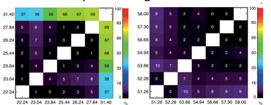
**Figure 9.** Percentage of tested days (268) in 2013 where the difference of TB pairs in the K band (left) and V band (right) are not within the calculated 2-sigma range (see Fig. 8).
