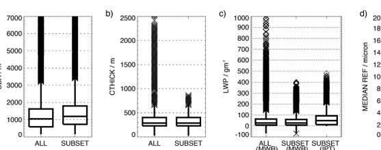
**Figure 12.** Boxplots of cloud base height (a), geometrical cloud thickness (b), LWP (c) and median REF of cloud profile (d) for all single-layer non-drizzling water clouds (SL WC) in 2013 (ALL) and for the SL WC subset captured by the IPT (SUBSET).
