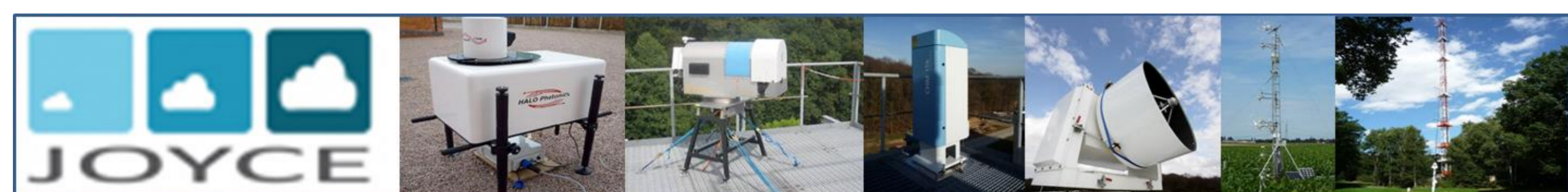
Fig. 1: JOYCE Instruments (left to right): Doppler lidar, Microwave Radiometer, Ceilometer, Cloud Radar, 120 m Meteorological Tower and Eddy Covariance station
