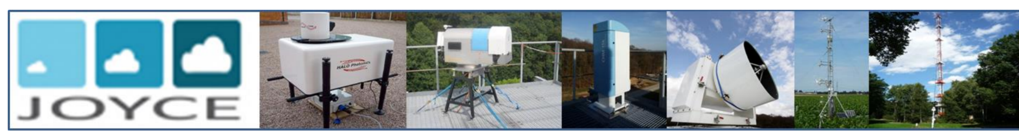
Fig. 2: JOYCE Instruments (left to right): Doppler Lidar, Microwave Radiometer, Ceilometer, Cloud Radar, 120 m Meteorological Tower and Eddy Covariance station
