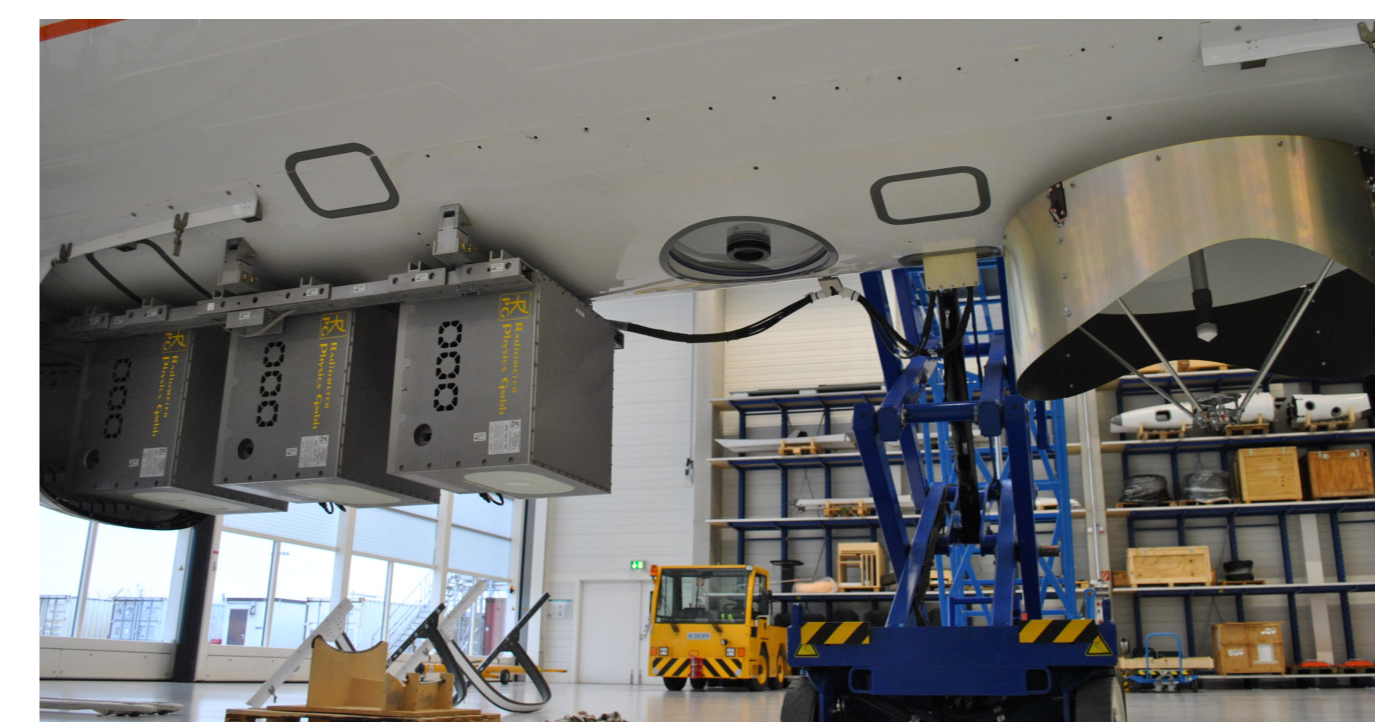
Fig. 3: Remote sensing suite on HALO. From left to right: radiometer boxes, lidar and radar.
