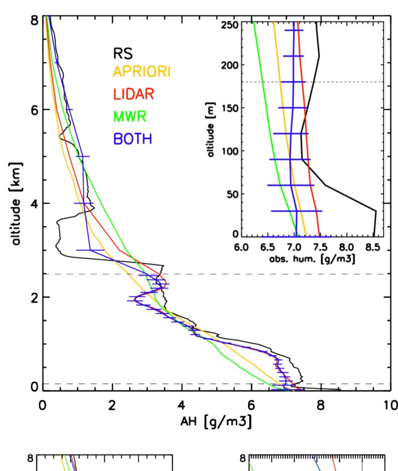
Top: AH retrieval for a single profile, on the 24th of April 2013 at 11 UTC and a zoom to the lowest 250 meters. Bottom: Example of temperature profile on the 17th of April 2013, at 23 UTC (a) Complete tropospheric profiles of temperature (b) Bias to the radiosonde and (c) zoom into the lowest 2km of the atmosphere. Measurements taken at JOYCE.
