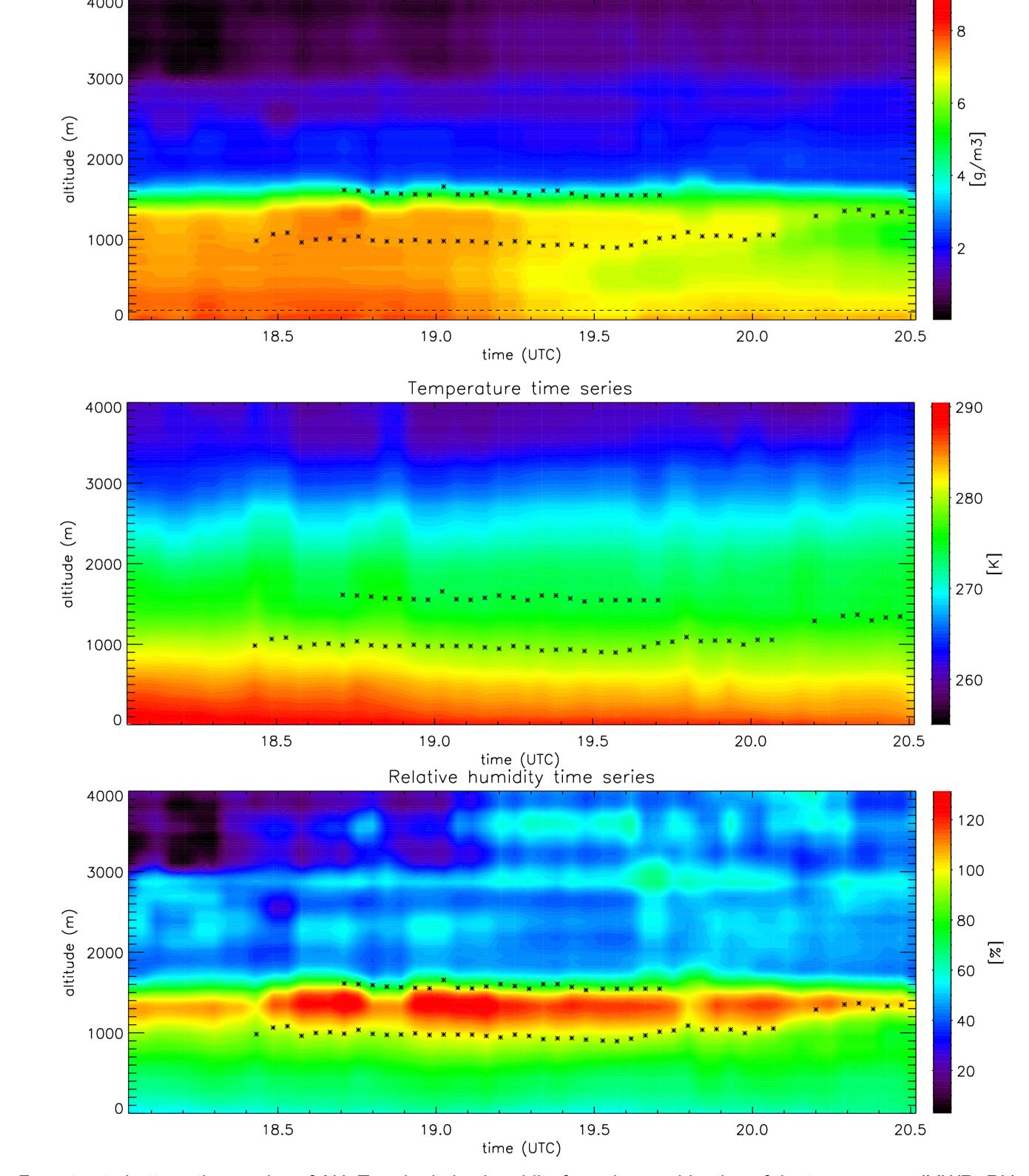
From top to bottom: time series of AH, T and relative humidity from the combination of the two sensors (MWR+RL). The period corresponds to the 4<sup>th</sup> of May 2013, from 18 to 20.5 UTC at JOYCE. The black dots represent the cloud base and top from ceilometer and radar, respectively.
