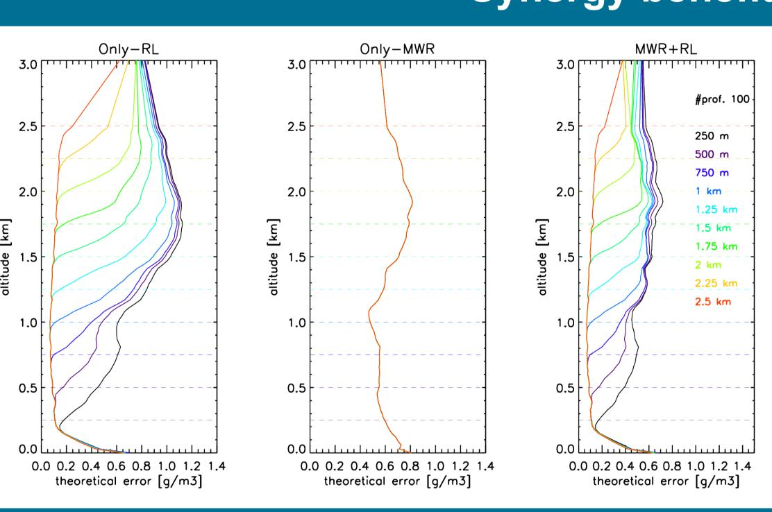
From left to right: average theoretical error for only-RL, only-MWR and MWR+RL, over 100 clear sky profiles, in the months of April and May 2013. Each colour represents a different clipping altitude (horizontal dashed lines) where lidar has been artificially cut.
