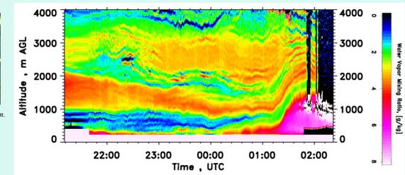
Fig.10. University of Hohenheim water-vapor DIAL measurement during August 1-2, 2007 (IOP13). At 0:10 UTC the approach of an outflow boundary ahead of cold front was observed in detail with resolutions of 10s and 300m, respectively. The moist layer at 3000 m was advected from the Mediterranean and embedded in a Saharian dust outbreak.
