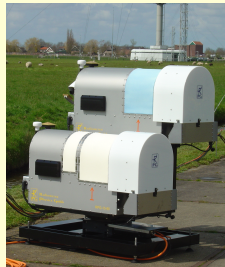
Master - Slave system: Master: HATPRO (top) Slave: 15 / 90 GHz
