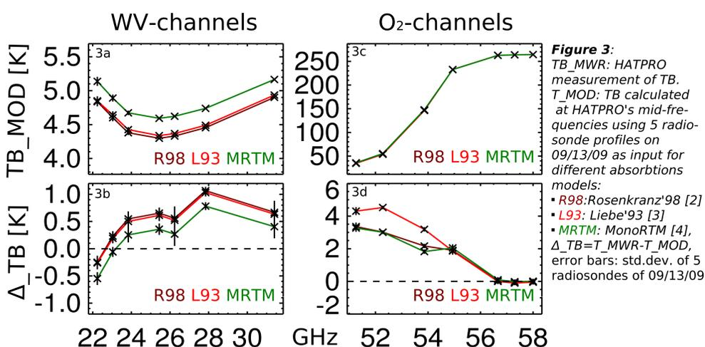
Figure 3: TB\_MWR: HATPRO measurement of TB. T\_MOD: TB calculated at HATPRO's mid-frequencies using 5 radiosonde profiles on 09/13/09 as input for different absorption models: R98:Rosenkranz'98 [2], L93: Liebe'93 [3], MRTM: MonoRTM [4], Δ\_TB=T\_MWR-T\_MOD, error bars: std.dev. of 5 radiosondes of 09/13/09
