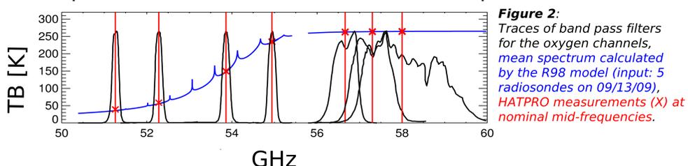
Figure 2: Traces of band pass filters for the oxygen channels, mean spectrum calculated by the R98 model (input: 5 radiosondes on 09/13/09), HATPRO measurements (X) at nominal mid-frequencies.
