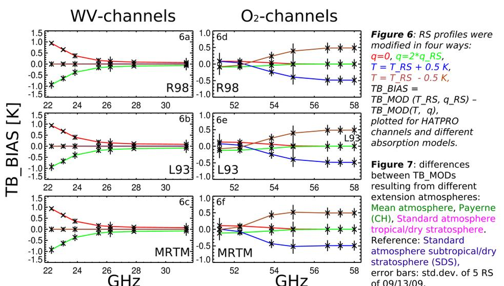
Figure 6: RS profiles were modified in four ways: q=0, q=2\*q\_RS, T = T\_RS + 0.5 K, T = T\_RS - 0.5 K, TB\_BIAS = TB\_MOD(T\_RS, q\_RS) - TB\_MOD(T, q), plotted for HATPRO channels and different absorption models.
