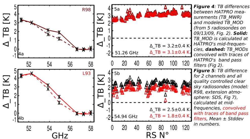
Figure 4: TB differences between HATPRO measurements (TB\_MWR) and modeled TB\_MOD (from 5 radiosondes on 09/13/09, Fig. 2). Solid: TB\_MOD is calculated at HATPRO's mid-frequencies, dashed: TB\_MODs convolved with traces of HATPRO's band pass filters (Fig. 2).
