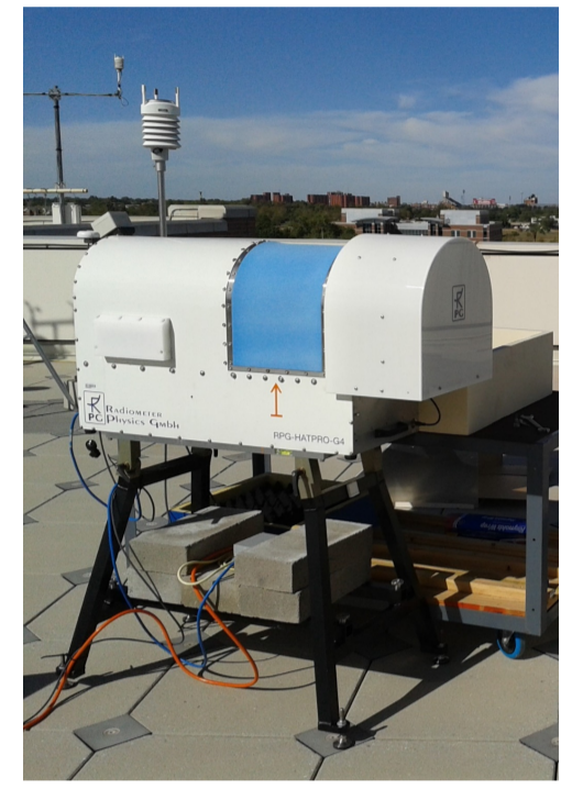
Fig. 1: HATPRO at the NSSL, Oklahoma, USA.
