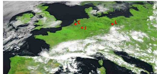
Fig. 1: RGB composite of Meteosat-8 SEVIRI's 0.6, 0.8 and 1.6 \mu\text{m} channels on 2 June 2011 (12 UTC) for the domain of interest. The brightness temperatures at 10.8 \mu\text{m} have been used as an additional weighting factor. The red dots indicate the location of the supersites Cabauw (C), JOYCE (J), and Lindenberg (L), for which the IPT will be applied.
