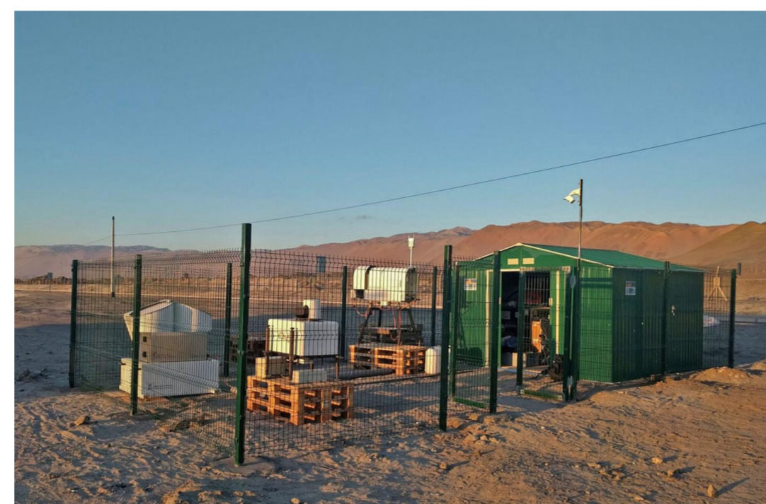
Fig. 1: Instrumentation at the airport of Iquique (20.5°S, 70.2°W, 56m AMSL). Instruments from left to right: cloud radar JOYRAD-94, wind lidar Halo Streamline (provided by the Finish Meteorological Institute (FMI)), microwave radiometer FOGHAT (AG Crewell, 2019).
