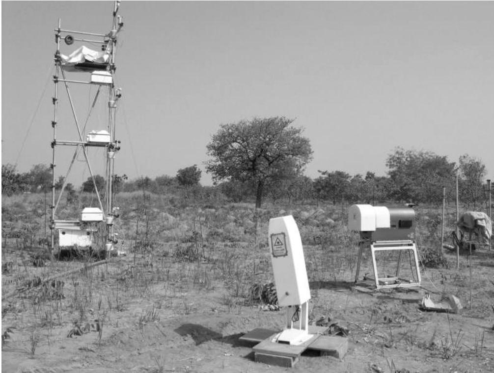
Figure 2. Setting of microwave radiometer HATPRO (right), lidar ceilometer (centre) and flux station (left) at the Nangatchori site in Benin.
