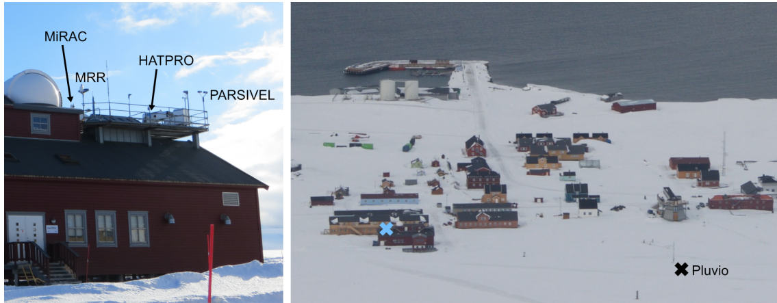
Figure 3.2: left: AWIPEV observatory, with remote-sensing instrumentation on the roof: Microwave Radar for Arctic Clouds (MiRAC, in the back), Micro Rain Radar (MRR), Humidity and Temperature Profiler (HATPRO) and laser-disdrometer PARTicle SIze VELOCITY (PARSIVEL); right: View from Zeppelin-Mountain (south-west) onto the village Ny-Ålesund and part of the Kongsfjord; blue cross: AWIPEV observatory; red cross: location of precipitation gauge Pluvio. Photo left: Kerstin Ebell, April 2017; Photo right: Pavel Krobot, April 2017
