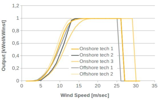
Power output as function of wind speed for different onshore and offshore technologies
