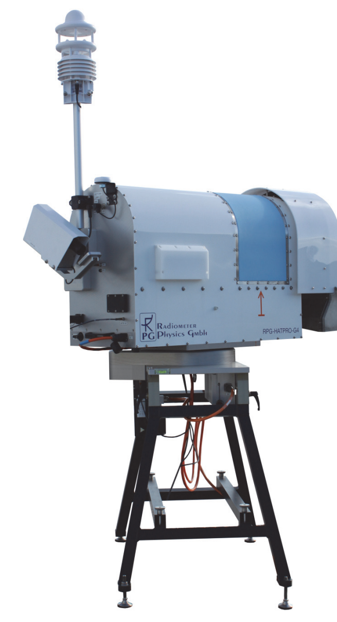
Hatpro (passive microwave radiometer): 7 channels at 22 GHz and 7 channels at 60 GHz.
