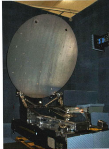
FIG. 5. The 2.5-m antenna for the 94-GHz radar.
