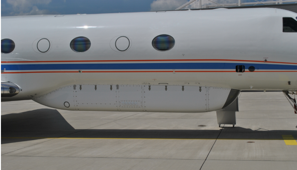
Figure 9: Belly pod on the bottom of HALO. Source: Mech et al. (2014) .
