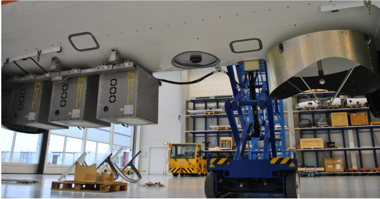
Figure 10: Instruments (left: MWR, consisting of three modules; middle: lidar; right: cloud radar) on the bottom of HALO, usually covered by the belly pod. Source: Mech et al. (2014) .
