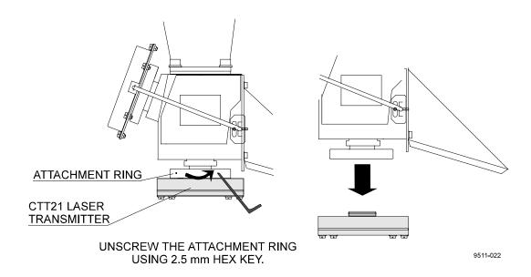
Figure 8-2 Removing the Laser Transmitter
