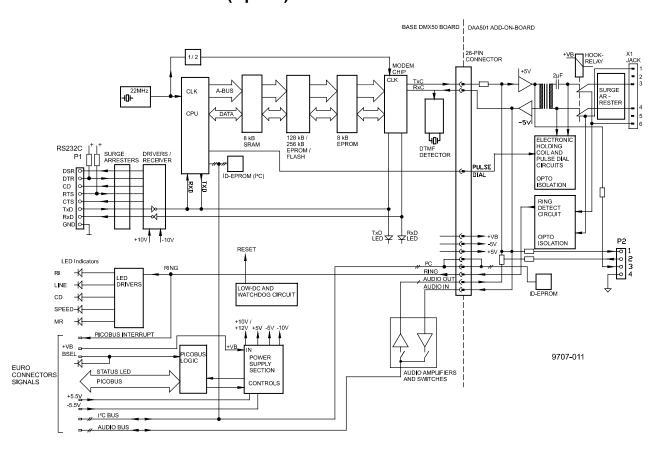
Figure 5-20 DMX50 Block Diagram
