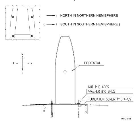
Figure 2-3 Mounting the Pedestal
