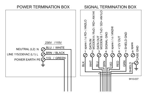
**Figure 2-6 Termination Box Wire Connections**
