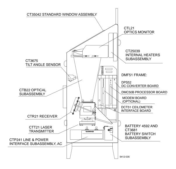
**Figure 5-2 Measurement Unit Components**
