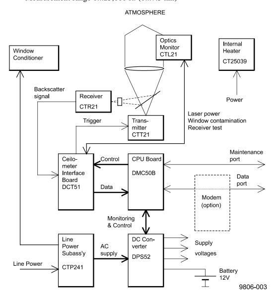
Figure 5-4 Block Diagram of Operational Units
