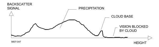
Figure 5-1 Typical Measurement Signal
