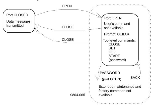
Figure 4-2 Open and closed port
