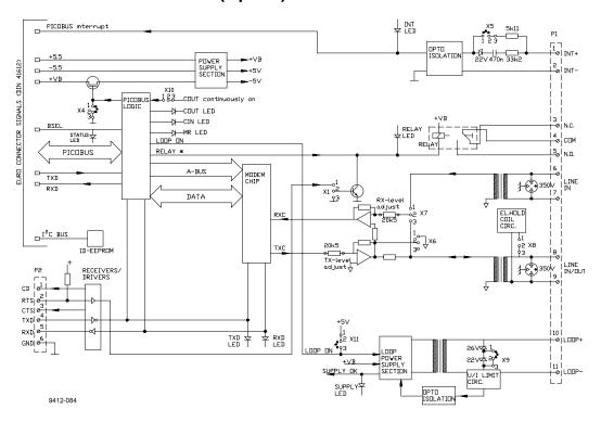
Figure 5-19 DMX55 Block Diagram
