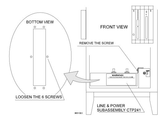
Figure 8-8 Removing Line and Power Interface Subassembly CTP241
