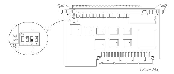
Figure 5-11 DIP Switch Settings of the DMC50
