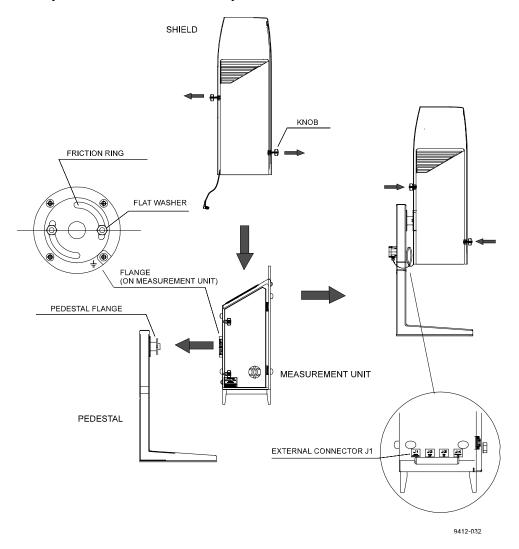
Figure 2-4 Attaching the Measurement Unit and the Shield
