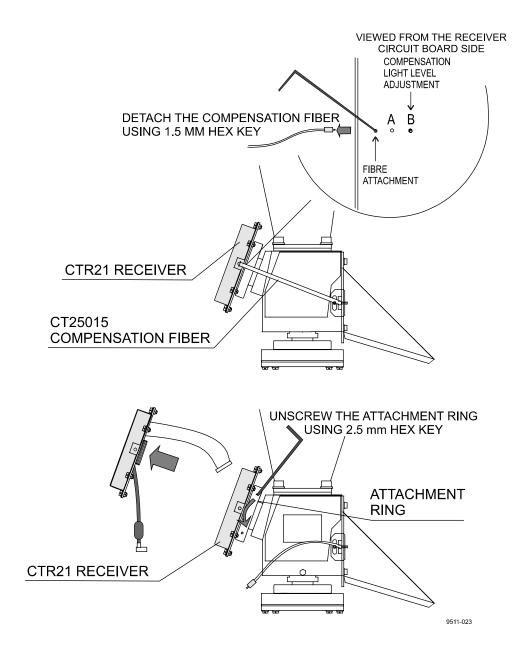
Figure 8-5 Removing the Receiver
