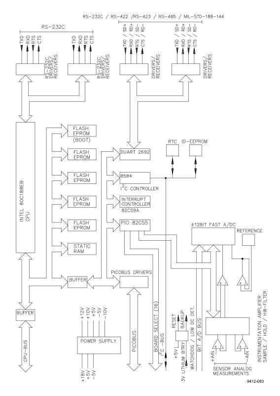
Figure 5-10 DMC50B Block Diagram
