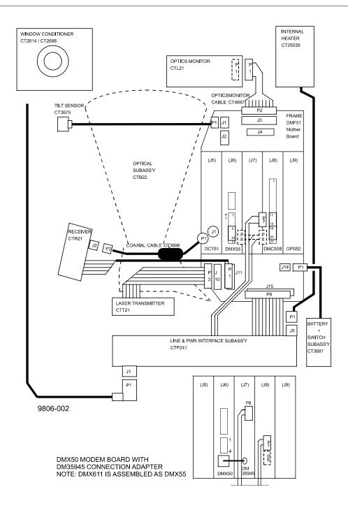
Figure 5-3 Subassembly Interconnections
