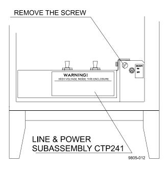
Figure 8-10 Battery replacement
