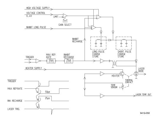
Figure 5-6 CTT21 Block Diagram
