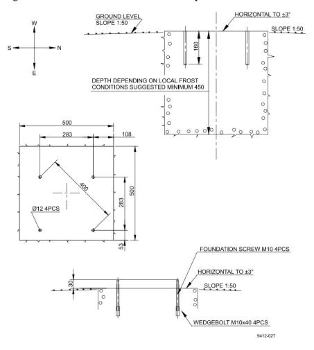
**Figure 2-2 Foundation Construction**
