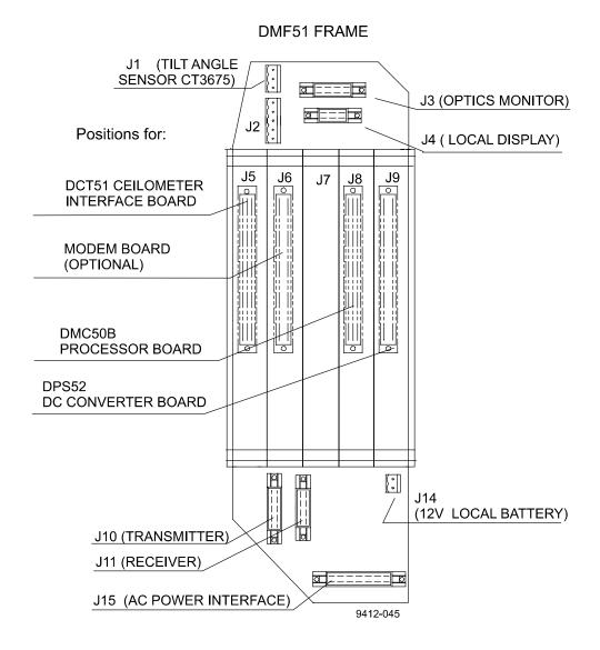
Figure 8-1 Board Connectors of the DMF51 Board Frame
