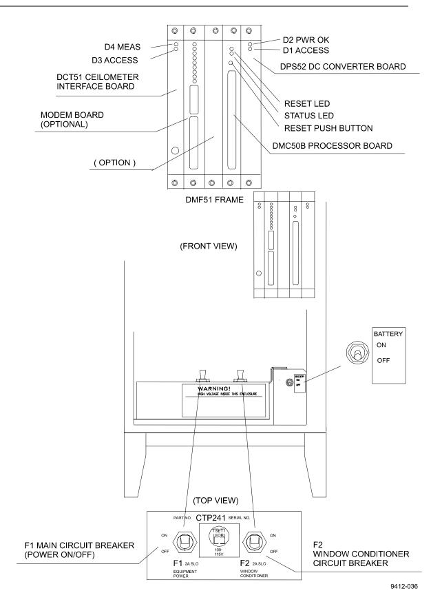
Figure 3-1 CT25K Switches and LEDs
