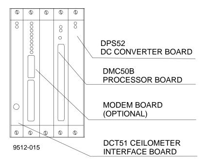
Figure 8-7 Boards of the DMF51 Board Frame
