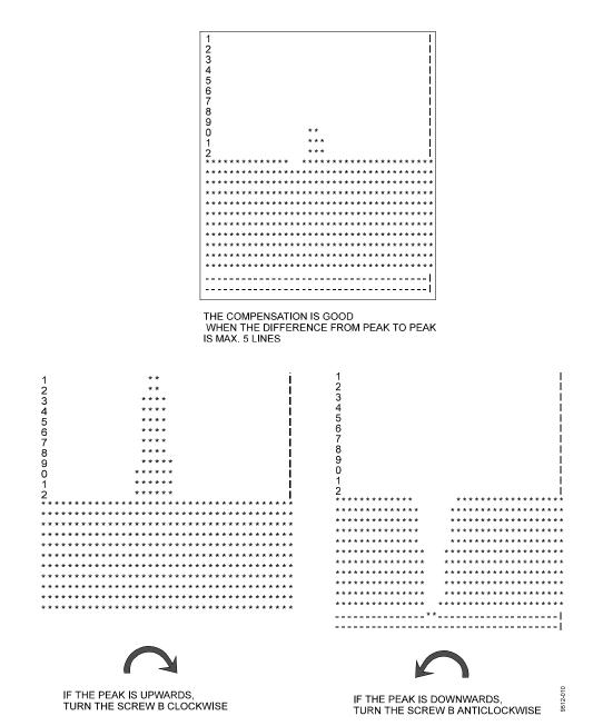
Figure 8-4 Adjusting the compensation
