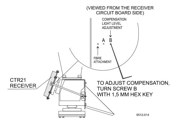
Figure 8-3 Adjusting the compensation
