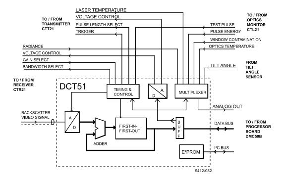
Figure 5-13 DCT51 Block Diagram
