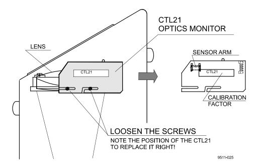
Figure 8-6 Removing the Optics Monitor
