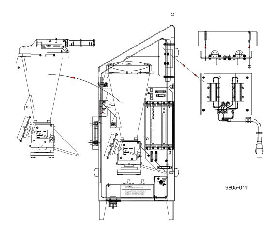
Figure 8-9 Internal heater replacement
