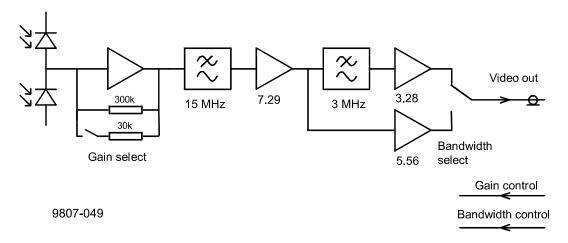
Figure 5-7 CTR21 Block Diagram
