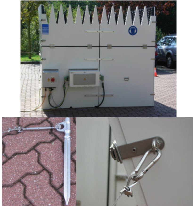
Figure 8: Fixture of the acoustic shields
