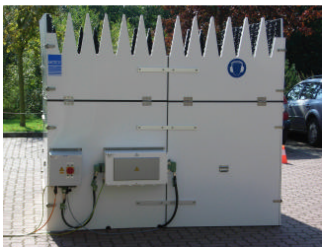
Figure 1: PCS.2000-64 with electronics in weatherproof outdoor cases
