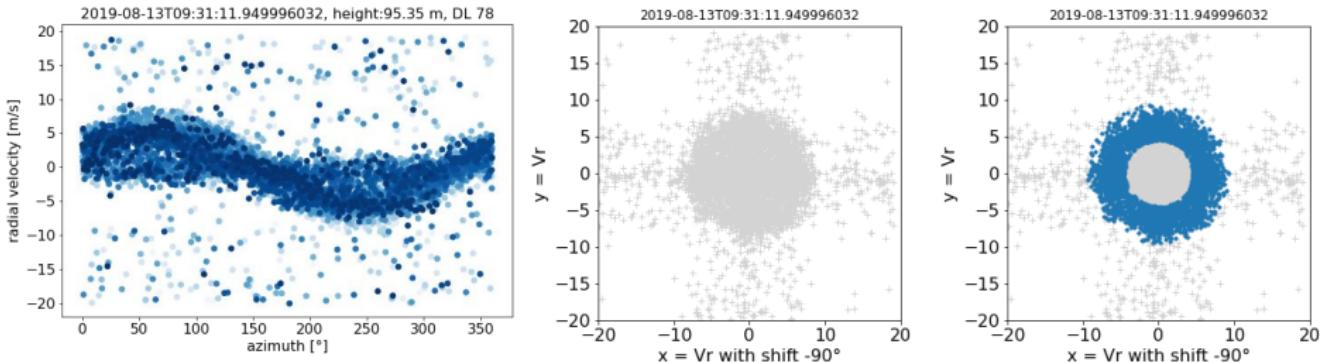
→ Use the auto correlation function (ACF) to identify radii bands around (0,0) without noise and discards the rest of the data.
