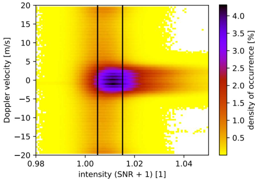
Left vertical line corresponds to an SNR value of -23 dB, right to -18.2 dB. Doppler velocities from 02/09/19 (25 mil. points).
