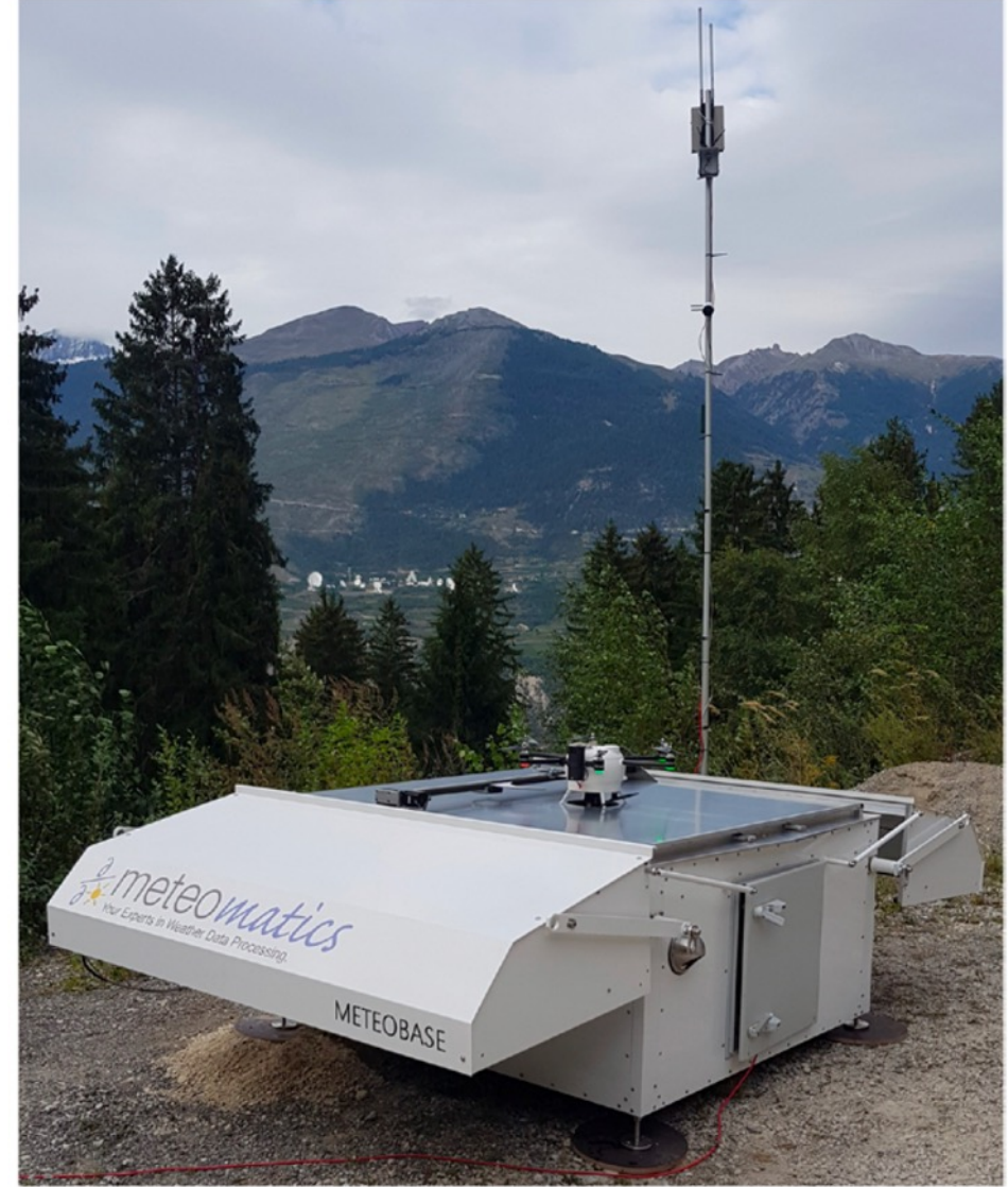
Fig. 5. Meteobase: The recently developed, fully automated launch and recharge system for the Meteodrones. The UAVs fly straight up, take their measurements, and land on the base for recharging via a connector.
